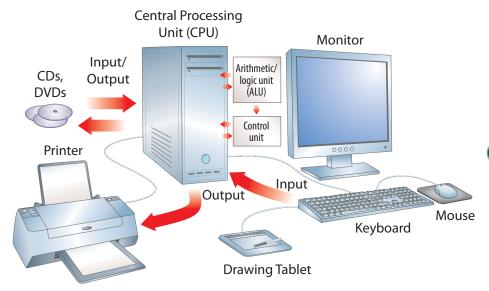
Plugging In A basic computer system includes the CPU, monitor, printer, keyboard, and other useful input and output devices.
